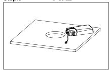
Put the driver into the opening of the ceiling and the driver installation complete.
