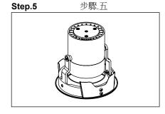
Press two side mounting clips direct to fixture and follow Step.6 into the ceiling.
