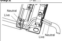
As shown in the figure, connect the live wire and neutral wire of the cable to the corresponding PRI slot in the driver.
