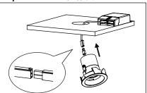
Connect the female connector and male connector, until you feel the connectors are lock.
