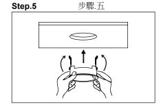
Push both the mounting clips of the embedded frame upwards and insert it into the cuthole on the ceiling.
