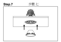
Insert the reflector into the fixture.
