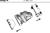
Remove the embedded frame and reflector from the fixture.
