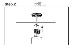
Connect the live wire, neutral wire and the earth wire of cable to the corresponding connector strip in the fixture.
