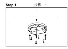
Pass the cable wire through the hole of the mounting part and tighten the part on the ceiling.
