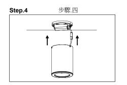
Connect the female connector in the driver with the male connector in the fixture.
