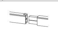
Connect the female connector and male connector, until you feel the connectors are lock.
