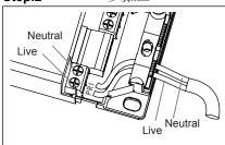
As shown in the figure, connect the live wire and neutral wire of the cable to the corresponding PRI slot in the driver.
