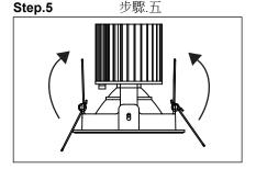
Press both sides mounting clip push up to the heatsink.
