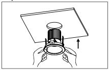
The whole fixture into the cuthole on the ceiling.
